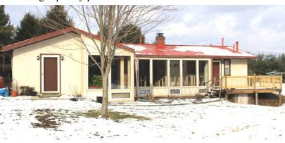
The deck on the house has been rebuilt, this time using recycled plastic lumber. Recycled plastic lumber finds a new use for discarded plastic while also providing a highly weather-resistant building material, perfect for outdoor locations.
